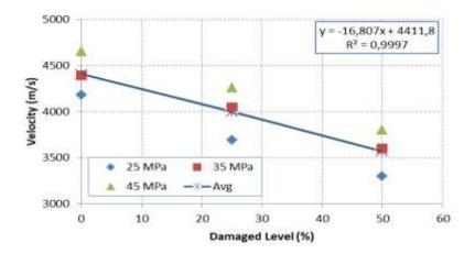
A regression is proposed in this research to predict the ultrasonic pulse velocity in reinforced damaged concrete based on experimental result
